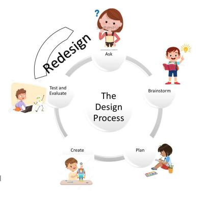
Industrial engineers use the Engineering Design Process to solve problems. The steps include:
